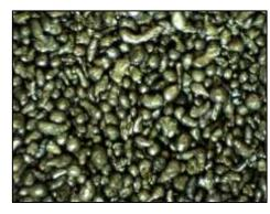
shorter processing times, better service life, and does not cause excessive machine wear unlike aluminium, corundum, and other ferrous steel media. This makes it perfect for cleaning, etching and cosmetic finishing, and for use in aluminum foundries, copper and alloy foundries, and in the iron and steel industry for stainless steel manufacturing. It is harder and therefore more suited to mechanical applications.
