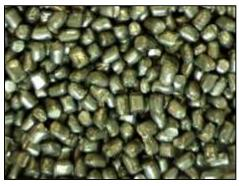
Typical Applications: Cleaning; cleaning of weldments; tumble blasting.
