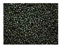
**Typical Applications (without dimensional changes to components):** Removing heat treat scale from components and sintered powder metal parts; cleaning of extrusion dies; cleaning of glass molds; cleaning of tire molds; de-flashing of delicate components; removing corrosion from machined surfaces
