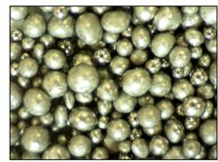
**Typical Applications:** Cleaning aluminum and nonferrous casting as well as forgings; peening; removing of heat-treating scale; surface preparation.
