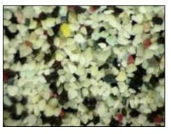
Typical Applications: Rust removal; light deflashing; removal of paint, anti-corrosions coatings
