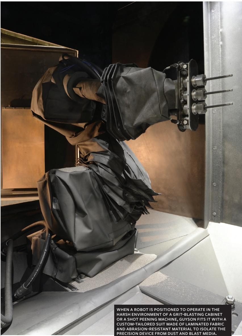
WHEN A ROBOT IS POSITIONED TO OPERATE IN THE HARSH ENVIRONMENT OF A GRIT-BLASTING CABINET OR A SHOT PEENING MACHINE, GUYSON FITS IT WITH A CUSTOM-TAILORED SUIT MADE OF LAMINATED FABRIC AND ABRASION-RESISTANT MATERIAL TO ISOLATE THE PRECISION DEVICE FROM DUST AND BLAST MEDIA.
